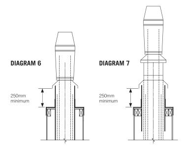
Option 2 - ECO Built-In flue kit with additional air supply vent (Diagram 7)
