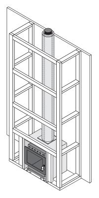
**STAGE 4**ECO Built-In flue kit assembly and installation
