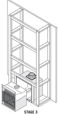
Insert firebox preparation and installation into the VZCC
