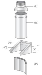
Dependent on whether you are installing into a flat roof/ ceiling or sloping ceiling situation as detailed on page 2, will determine if you require all the components of the ECO Option Kit. If installing into a flat ceiling/roof you will not require the drop box or drop box edge covers.
